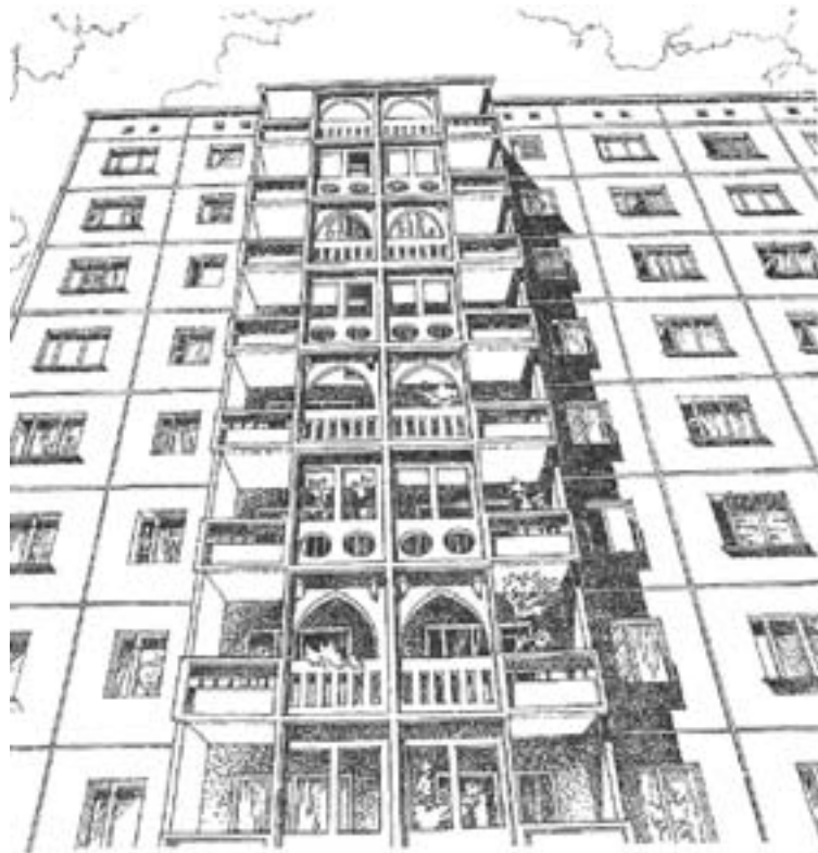
FIG. 12. Tashkent. Prefabricated decorative elements of a residential building. Architects: A. Kosinsky, V. Azimov and others. (Source: TashGiprogor.)
