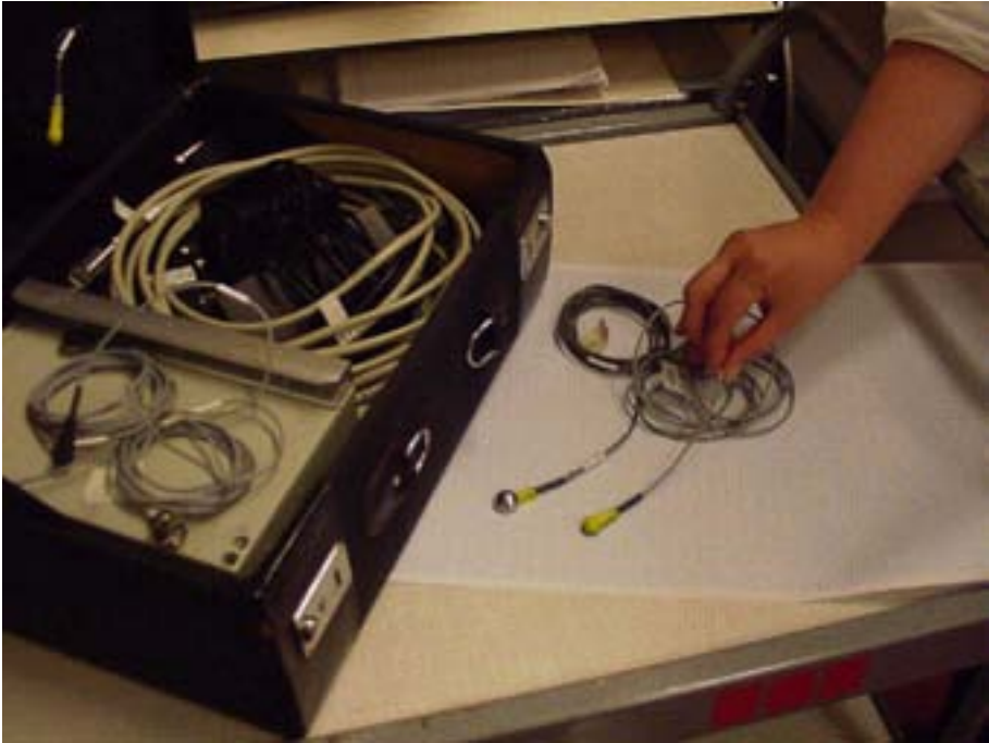
FIG. 12.4. Diodes applied for in vivo dosimetry.
