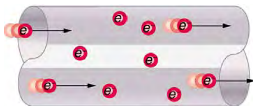
Figure 20.5 When charged particles are forced into this volume of a conductor, an equal number are quickly forced to leave. The repulsion between like charges makes it difficult to increase the number of charges in a volume. Thus, as one charge enters, another leaves almost immediately, carrying the signal rapidly forward.
