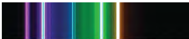
Hg vapor spectrum (350-700 nm)
