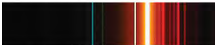
Low-pressure Na spectrum (350-700 nm)
