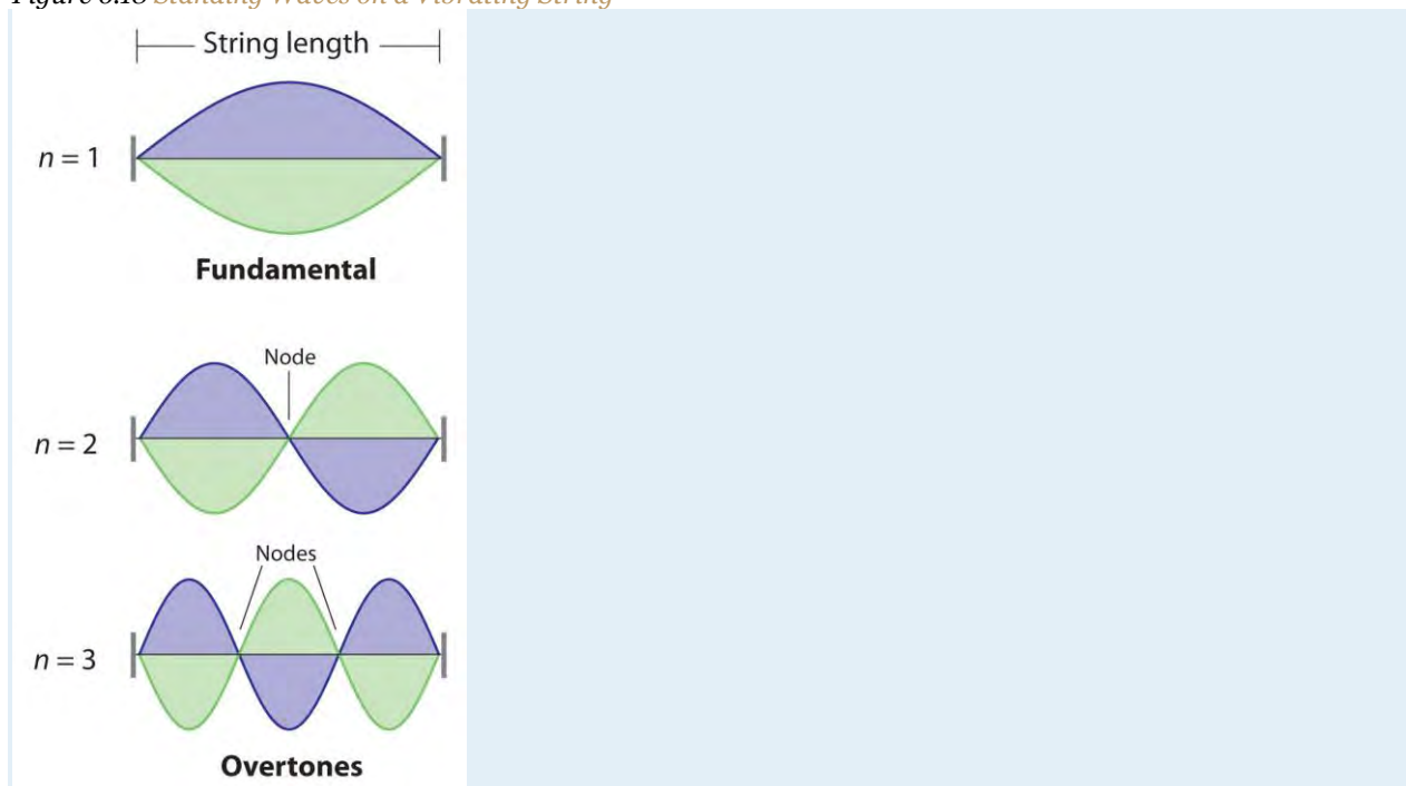
Figure 6.18 Standing Waves on a Vibrating String
