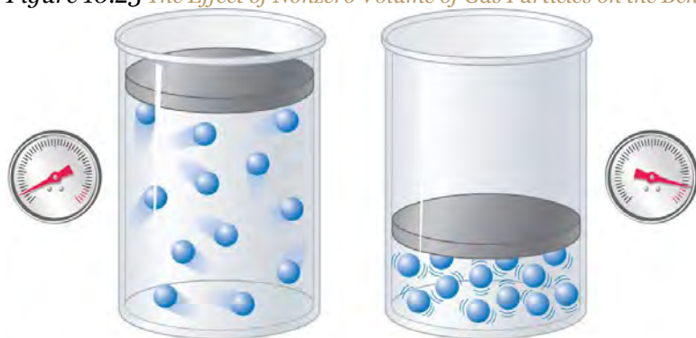
Figure 10.23 The Effect of Nonzero Volume of Gas Particles on the Behavior of Gases at Low and High Pressures
