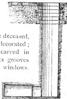
Fig. 138.—Section showing shaft and vault of mastaba at Gizeh, Fourth Dynasty.
