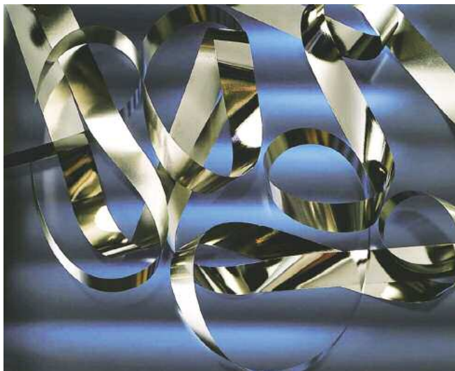
Nanocrystalline blank tape with a thickness of only 18 \mu\text{m} as basic material for optimized inductive components (source: Hitachi Metals Europe©)
