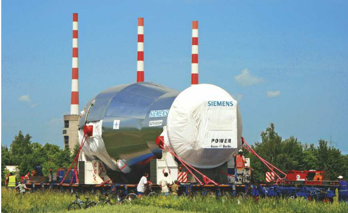
The world's largest gas turbine with a capacity of 340 MW installed in a power plant in Irsching which began trial operation at the end of 2007. The overall efficiency of the power plant is stated to be approx. 60% (source: Siemens).
