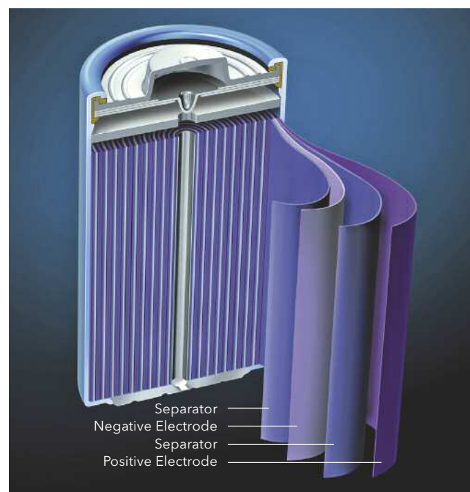
Basic structure of lithium-ion batteries (source: Evonik)
