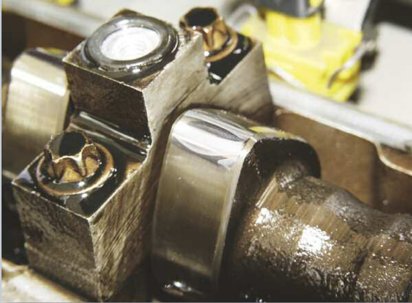
The picture shows the wear-protection coating of a camshaft. The strongest coating occurs in the area exposed to the highest pressure at the highest point of the cam.
