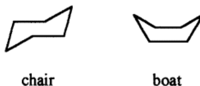
Figure 3.13. Chair and boat conformations of cyclohexane
