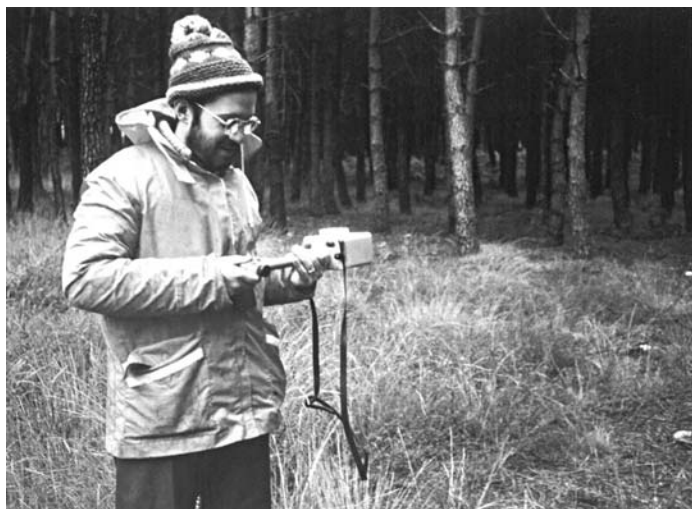
Figure 9.7 Searching for the station with the EM-16.
